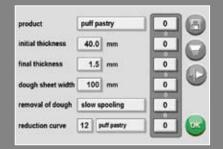
Here's how easy it is to set up a dough sheeting program for a specific dough type: via a standard computer keyboard you call up the name of the product onto the monitor and then enter the beginning and final
