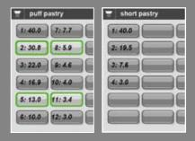
In this detailed view of the individual dough sheeting reduction curves, you see not only the number and sequence of the dough sheeting steps but also with the help of the green highlighting at which stage of sheeting the flour duster is switched on.
