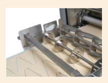
This regulator allows for the appropriate control of the belt speed for dough cutting or a dough transfer of 2 - 7 m/min.
